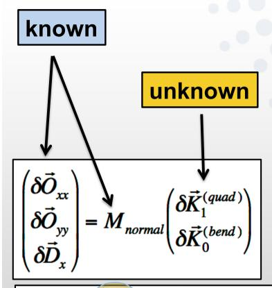
$$ORM = \begin{pmatrix} O_{xx} & O_{xy} \\ O_{yx} & O_{yy} \end{pmatrix} \longrightarrow Orbit \quad \text{Re sponse Matrix}$$
