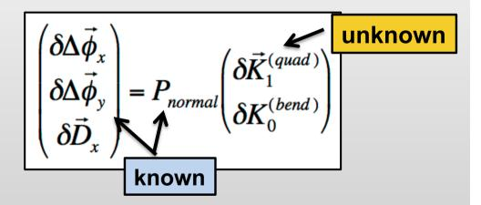
this linear system can be pseudo-inverted via Single Value Decomposition (SVD) to infer quad & bend field errors  $\delta K_0 \& \delta K_1$
