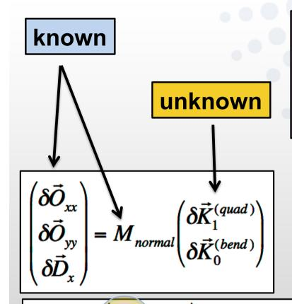
this linear system can be pseudo-inverted via Single Value Decomposition (SVD) to infer quad & bend field errors  $\delta K_0$  &  $\delta K_1$
