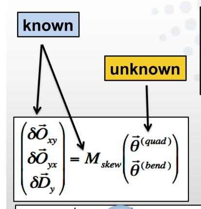
this linear system can be pseudoinverted via Single Value Decomposition (SVD) to infer quad & bend tilts &(quad) & &(bend)
