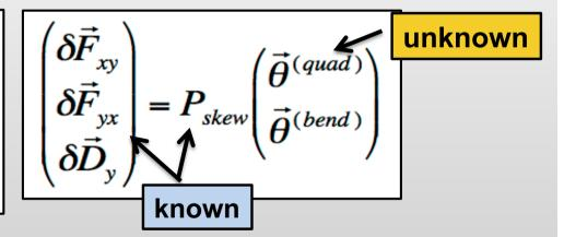
this linear system can be pseudoinverted via Single Value Decomposition (SVD) to infer quad & bend field tilts ϑ(quad) & ϑ(bend)
