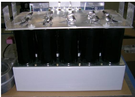
SR Dipole PS: Redesigned DC link capacitor banks ⇒ 120 000 hours
