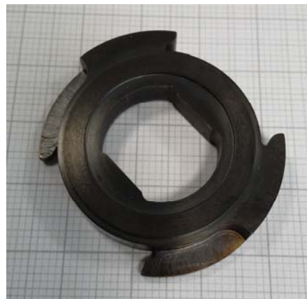
Figure 6: The actuation claw. The single blade actuation claw is to bottom left, while the three blade option is to top right. This item is DLC coated.
