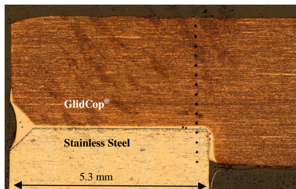
Figure 3: Stainless steel to GlidCop ® vacuum braze.
