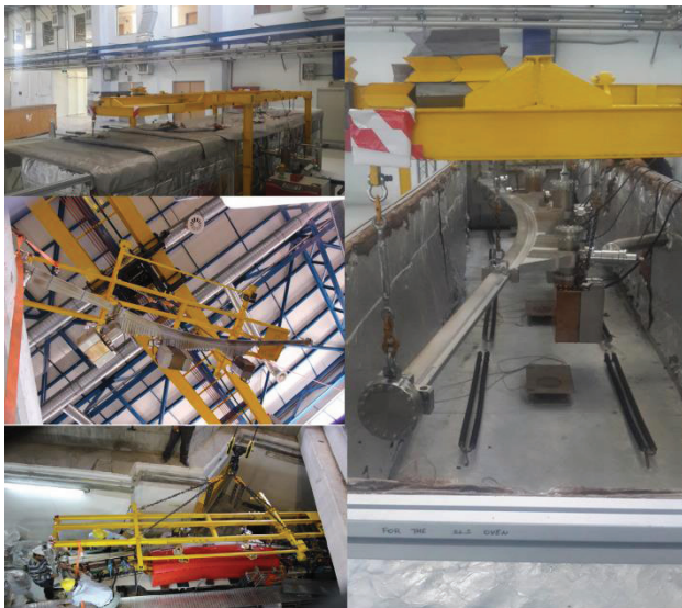
Figure 8: A photos during the assembly, bake-out and installation of the storage ring vacuum chambers.
