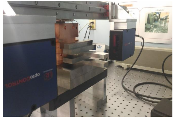
Figure 5: Receiver sensor with gauge block gap calibration.
