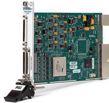
Figure 5: The picture of FPGA Module.
