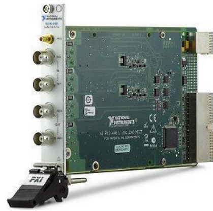
Figure 4: The picture of high-accuracy data acquisition devices.
