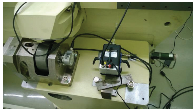
Figure 6: A shaker to simulate the vibration source.
