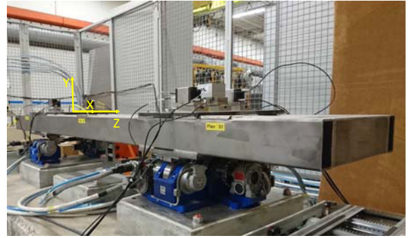
Figure 2: Type 4 MBQ and stabilisation system mounted on cam movers (left) and test setup including ZCMs, follower girder and local coordinate system (right).
