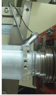
Figure 1: cooling pipe of vacuum chamber.
