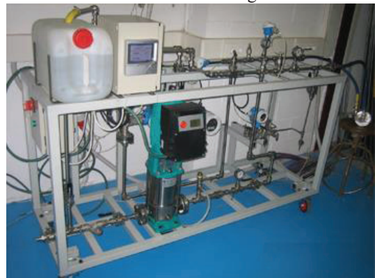
Figure 4: The ALBA experimental hydraulic unit to characterized pressure drop versus flowrate.
