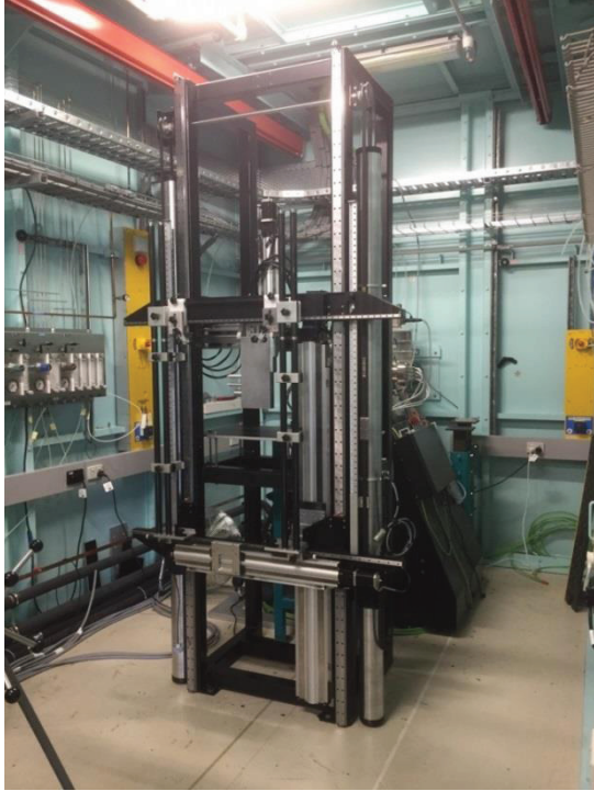
Figure 6: Milliprobe scanner station recently installed in XFM end station.
