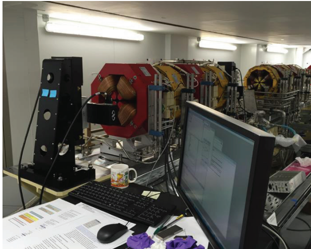
Figure 4: Stretched wire measurement of magnet groups.
