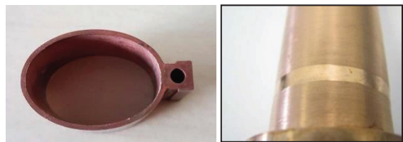
Figure 8: Full penetration welding of copper.
