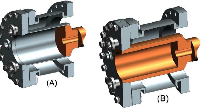
In order to enhance the heat dissipation on the air cooling system, three geometries are studied: A) Stainless steel cylinder, 2 mm wall thickness, B) Copper cylinder, 10 mm wall thickness, and C) Case B with internal fins attached.
