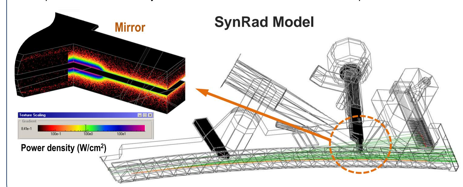
Surface power density distribution using the SynRad+ computer code.
