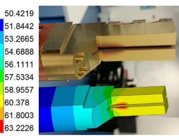
Case C. Included a real photo captured during the commissioning stage. The carbonized zone in the mirror matches the observed BM power deposition calculated by SynRad+. The local temperature measured in the body above the slot was 25.5 °C with 130 mA. The FEA model predicts a range < 32 °C.
