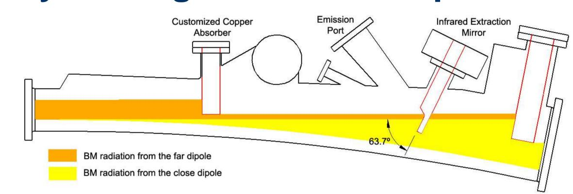
Ray tracing for MIRAS dipole chamber. The orange fan is the BM radiation coming from the far dipole chamber and the yellow zone is the radiation from the close dipole.
