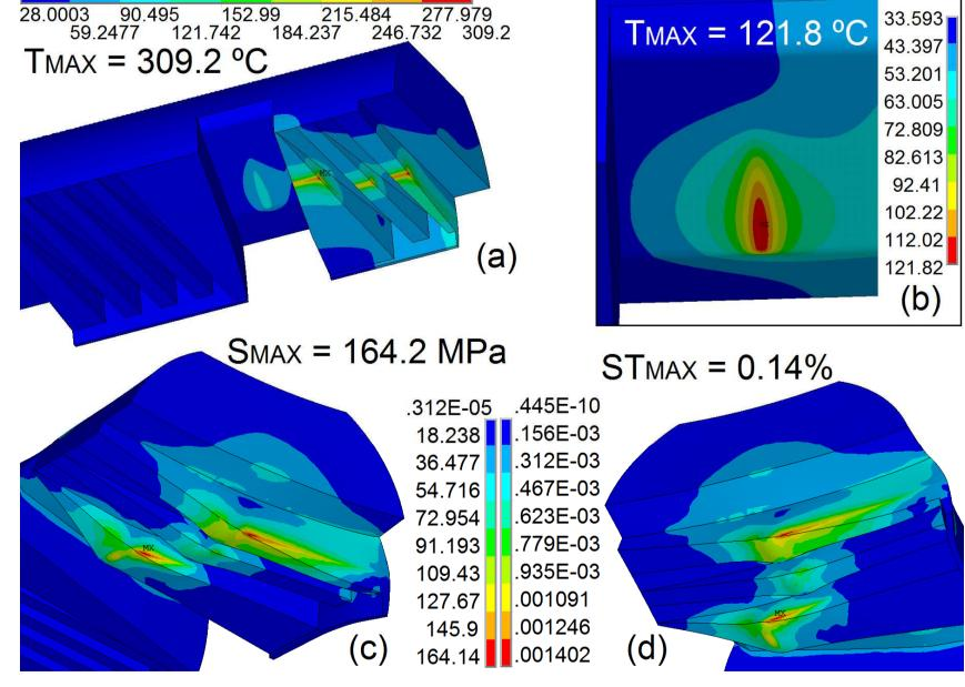
The temperature, stress and strain distribution have been calculated based on linear elastic analysis. The thermal mechanical simulations show good results, the new absorber is in a safe range according to the design criteria. The maximum temperature, stress and strain are 309.2 °C, 164.2 MPa and 0.14%, respectively.
