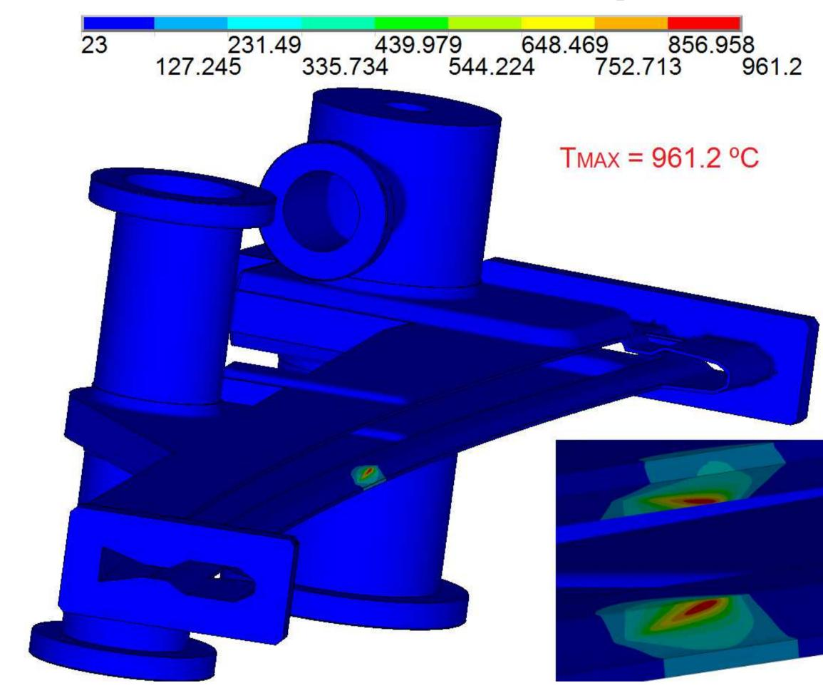
Temperature reached on the dipole chamber (upper and lower cooling channels) due to interference of ID radiation in vertical mode. The maximum temperature is 961.2 °C. The current working point of water has been imposed as boundary condition: h = 1500 W/m<sup>2</sup>K at 23°C.
