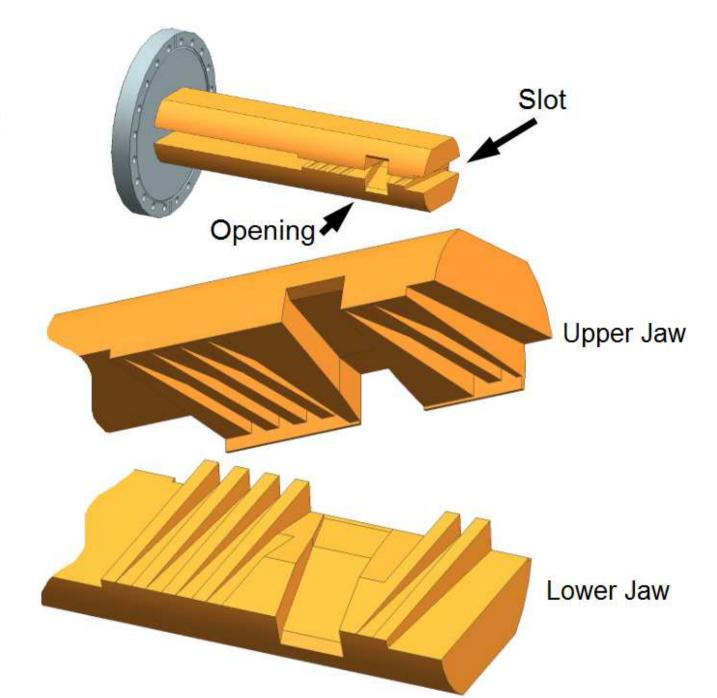
The assembly and two jaws of new Glidcop Al–15 crotch absorber for LOREA dipole chamber.
