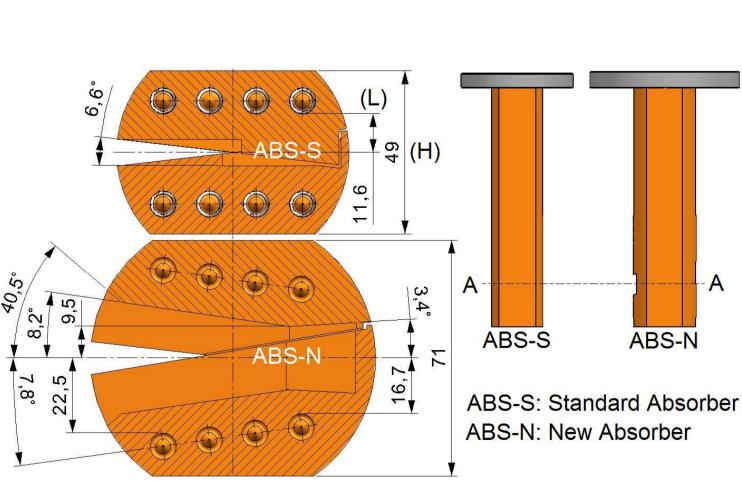
Comparative study between the dimensions of standard (ABS-S) and new crotch absorber (ABS-N). View for the cross section A–A. Dimensions are in mm.
