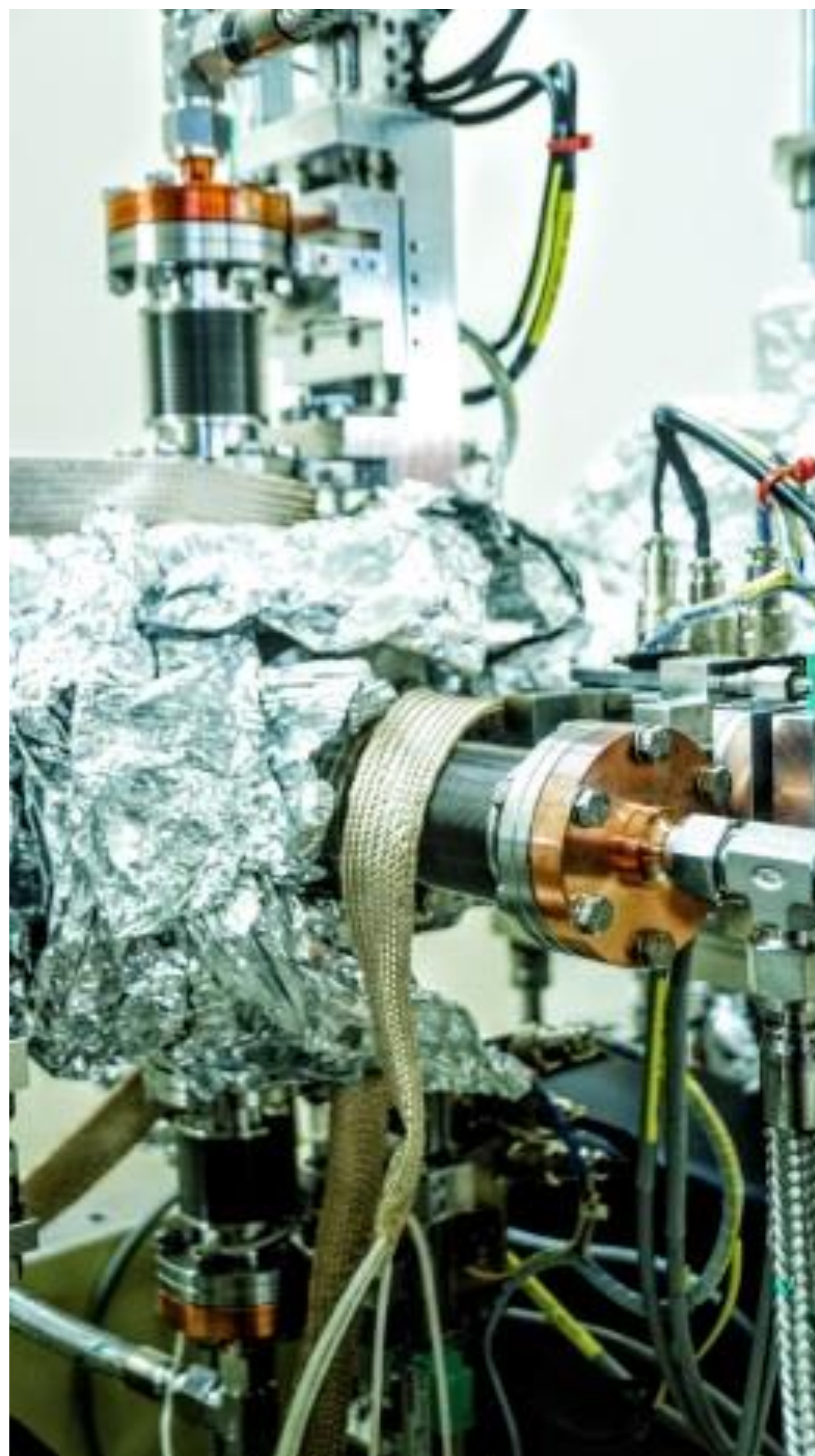
CuCrZr slits in TPS front end 24
