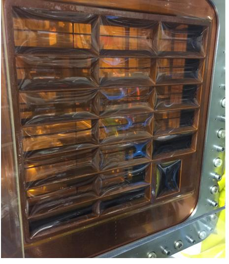
The parts were manufactured and assembled, and they went through a pressure test to check that there were no leaks or visible damage. A visual examination did not highlight any noticeable permanent deformation so the window is now operative; a test is planned to measure stress and strain, so the results can be compared to the simulated ones, to validate them.
