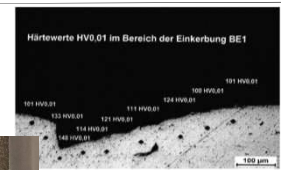
Polished cut image of DESY 72° knife edge contour
