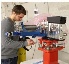
This picture show Max during the final assembling a type B chamber in the XFEL tunnel
