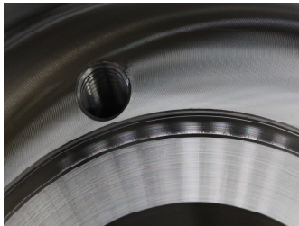
ISO/TS 3699-2 DESY standard knife edge
