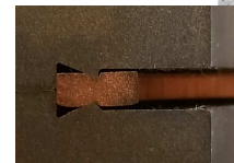
This picture is presented pairing of DESY knife edge with ISO/TS 3699-2 knife edge
