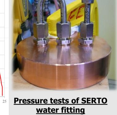
Static pressure test at 20 bars during 4 hours at 20° Dynamic pressure test at 10 bars during 24 hours at 20° New static and dynamic test after bake-out cycle at 200°
