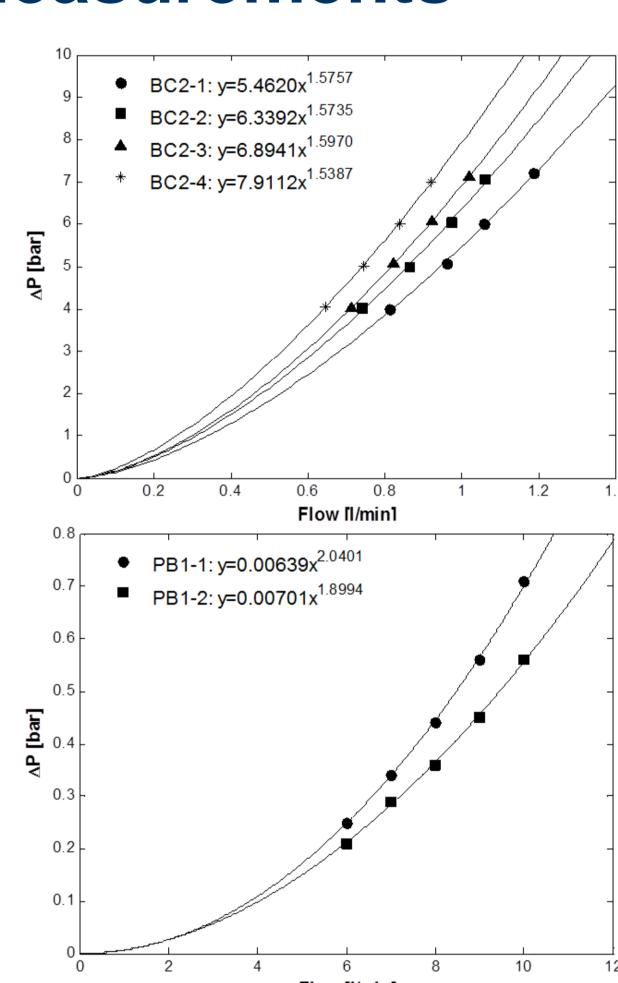
**Example case:** Pressure drop versus flowrate experimental correlations for BC2 and PB1.
