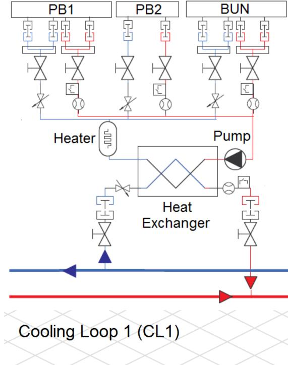
An accurate 1D model of the LINAC cooling system has been built. The model includes all the net pipes, bends, pipe entrance, changes of section, branding of current, valves (open/close type, regulators), pressure reducer, flowmeters, pumps and local components. A total of 199 pipes and 57 components have been used for the simulation model. The numerical predictions have been compared with experimental data. A good agreement has been found with deviations of the main variables below 11%.
