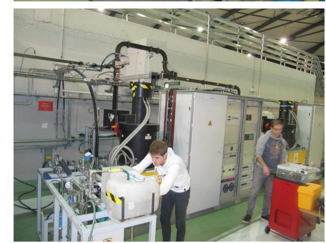
All the LINAC sub components have been characterized in terms of the pressure drop versus flowrate. The measurements were taken using a portable hydraulic unit as well as a set of ultrasonic flowmeters.
