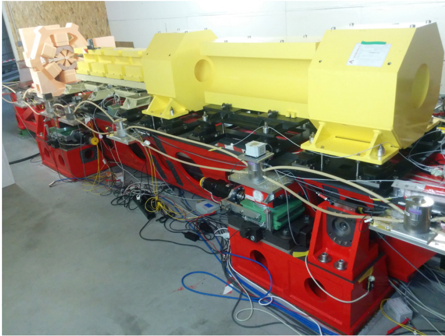
Full scale mock-up girder prototype with power cables inside Why cables inside the girder?
