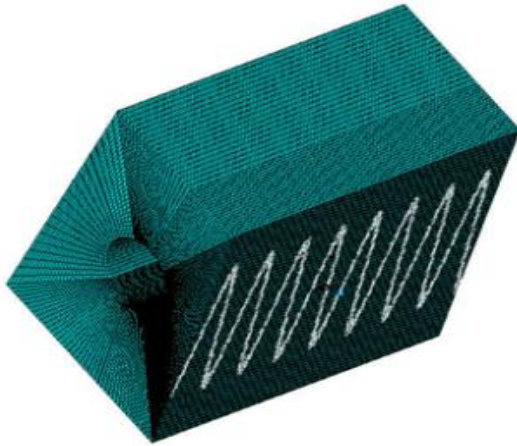
FE Model – Beam footprint from a Sine Wave Gap
