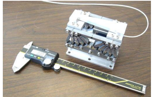
Figure 10: Photograph of the Z7-5006 prototype dynamic mirror bender with closed-loop control configuration.
