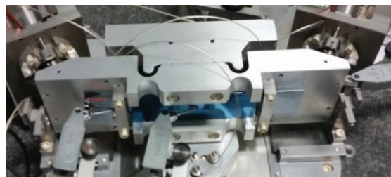
Figure 5: A prototype of the bender with its crystal. Two piezo-jacks behind are pulling/pushing on both sides. The path is free in the middle for the X-ray beam.
