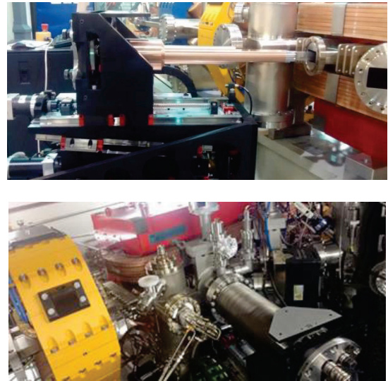
Figure 6: Top: Mechanics assembly mounted on mock-up girder. Down: Extraction mirror retracted mounted inside accelerator's tunnel.
