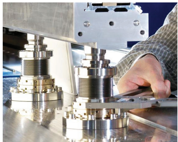
Figure 6: Adjustment of the columns.
