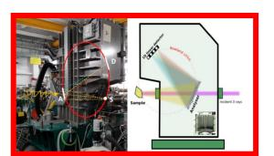
CLEAR spectrometer XES 20-30 min typical acquistion up to 23 keV K $\alpha$ , K $\beta$  emission lines 10min (K $\alpha$ ), 30-40min (K $\beta$ 1,3), 1-4h
