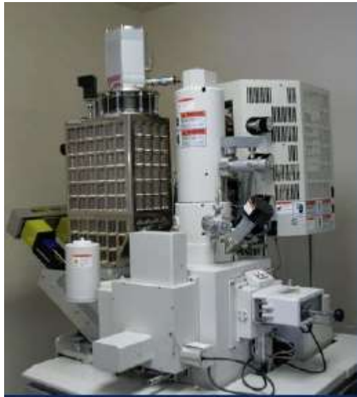
Commercial SEM-mounted cryogen-free spectrometer (16-TES array) from STAR Cryoelectronics
