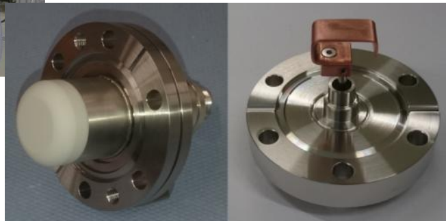
cavity probe: old design (left) and new ALBA design (right)
