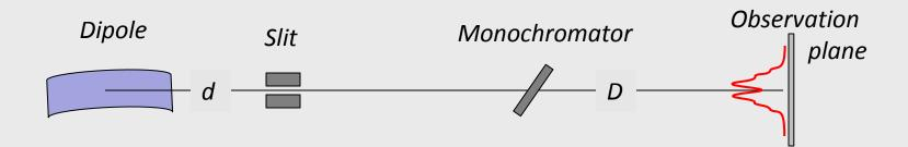
Optimum slit size for obtaining a « simple » double-lobed diffraction pattern [1]:
