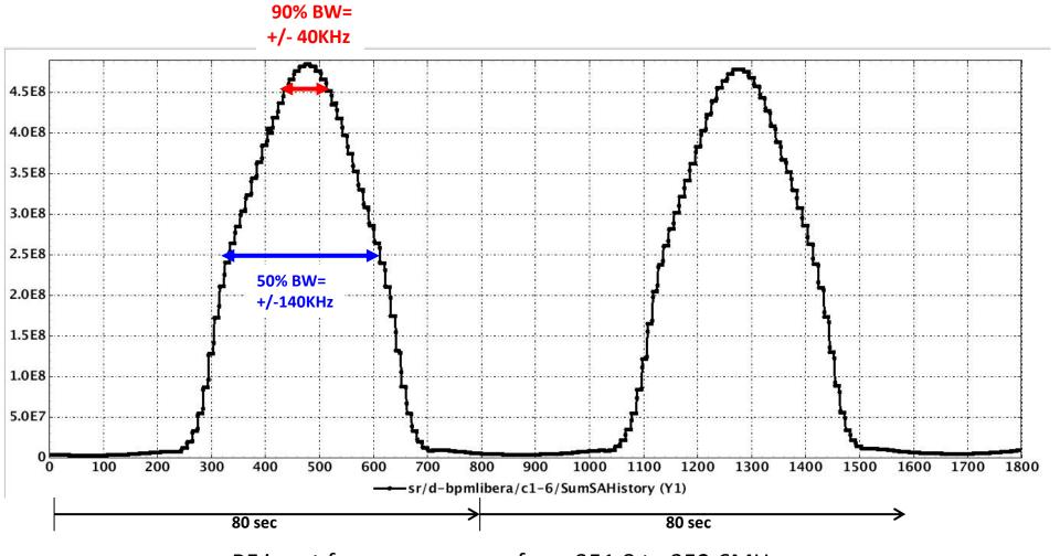
RF input frequency sweep from 351.8 to 352.6MHz, i.e. 352.2MHz +/- 400KHz, in 80 steps of 10KHz, at 1 sec interval Storage Ring Libera itself synchronized to 352.202 MHz/ 992 (MC)
