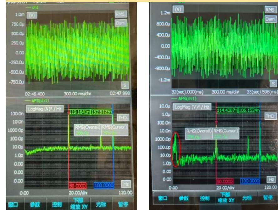
Power supply ripple of one SC with and without PWM frequency tuning
