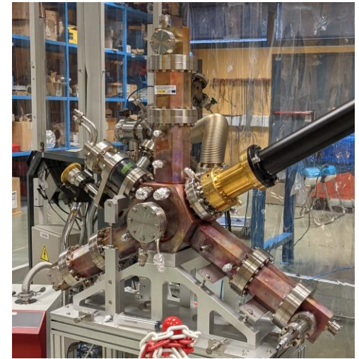
4x Harmonic NC active RF cavity prototype 170 kV - 1500 MHz
