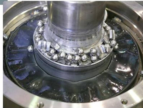
Cold Compressor 4 bearing failure
