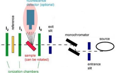
Fluorescence detector is set at 90 degrees respect to the incoming beam to minimize the scattering peak.
