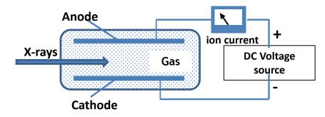
Inert gas mixture is chosen depending on the photon beam incoming energy
