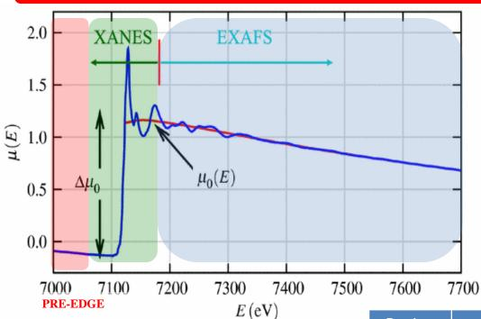
The measurement grid change as a function of the XAS spectral region:
