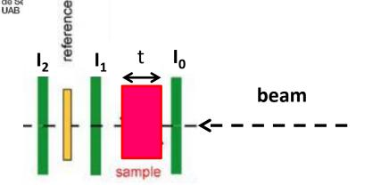
Lambert-Beer:  $I=I_0 e^{-\mu(E)t}$   $\mu(E)t=-\ln(I/I_0)$   $\mu(E)=x$ -ray absorption coefficient at energy E, t=t-thickness of the sample
