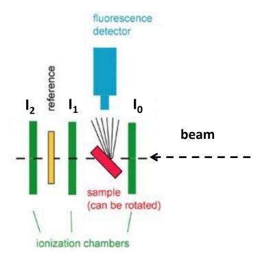
Measure the fluorescence X-rays I<sub>f</sub> that are emitted following the X-ray absorption event.
