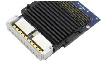
FMC LXD31K4-DC 4 channel 16-bit ADC/DAC (Logic-X )
