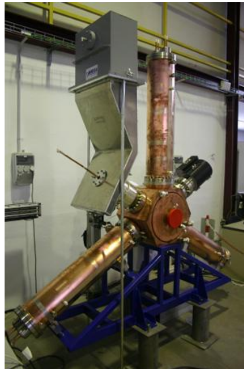
6x Main NC RF cavity 400 kV - 500 MHz
