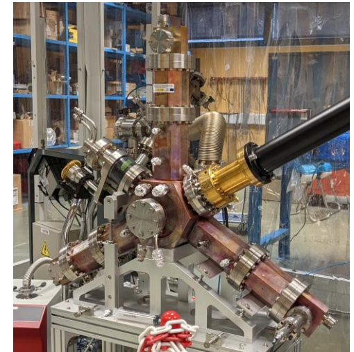
4x Harmonic NC active RF cavity 170 kV - 1500 MHz
