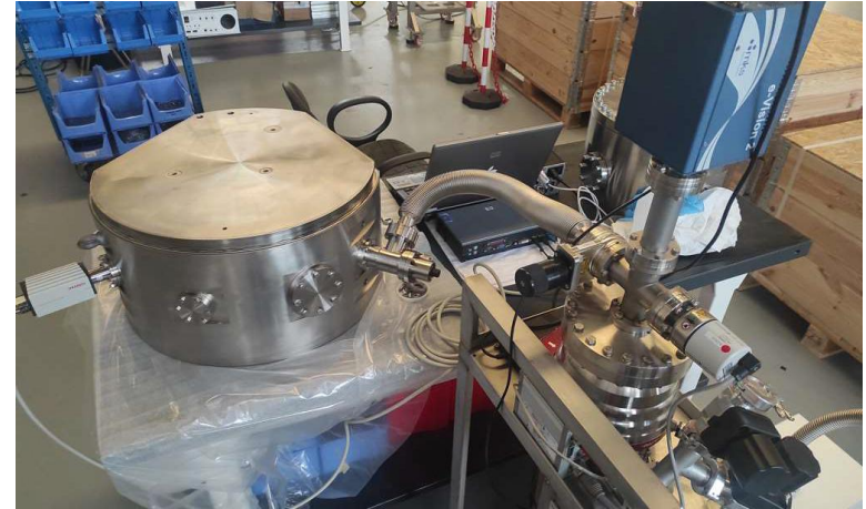
IC3 cavity being tested for leaks
