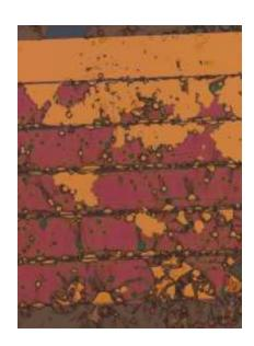
The E-beam flux is not perfectly stable + arcing possible that leads to spitting and particles on the substrate.
