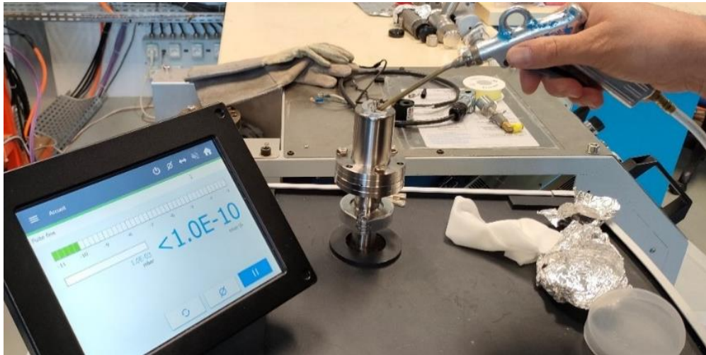
Helium leak test
