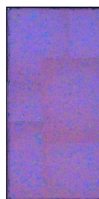
1.7 \mu\text{m} pyrolyzed film (1 layer)
