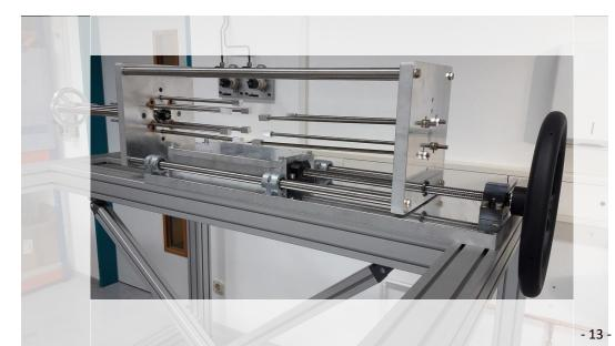
PM Measurements via 2D-Helmholtz-Coils
