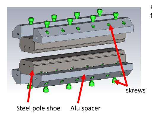
Pole shoes are fixed with the yoke in an Aluminum ( $\mu_r$ =1) framework
