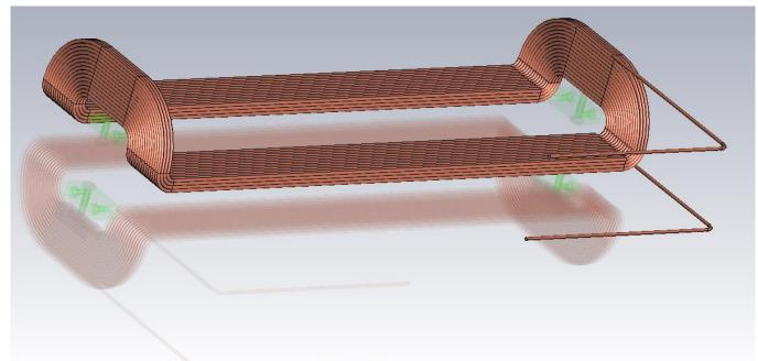
Flat corrector coils in the outer magnets for fast correction of the magnetic field (bending angle)
