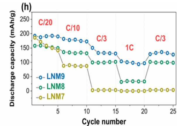
In-situ battery measurements using synchrotron and neutron diffraction
