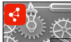
MicroElectroMechanical (MEMS) devices 10 -100 \mu\text{m} wide
