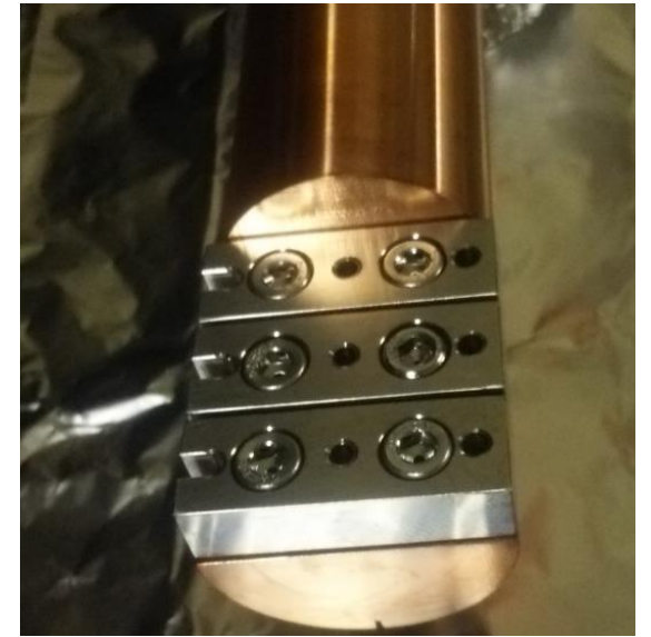
Water-cooled mask holder
