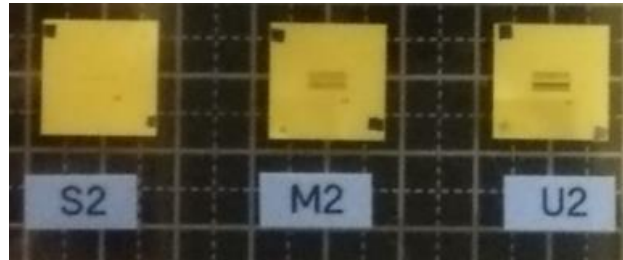
Masks: \sim 20\ \mu\text{m} Au on 600\ \mu\text{m} CVD diamond substrate
