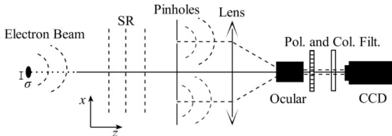
$$I = I_0 \left\{ \frac{J_1\left(\frac{2\pi ax}{\lambda f}\right)}{\left(\frac{2\pi ax}{\lambda f}\right)} \right\}^2 \times \left\{ 1 + V \cos\left(\frac{2\pi D x}{\lambda f}\right) \right\}$$
