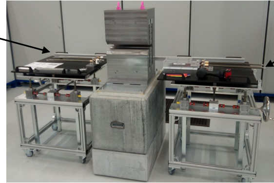
Assembly table mounted around the BN magnet.
