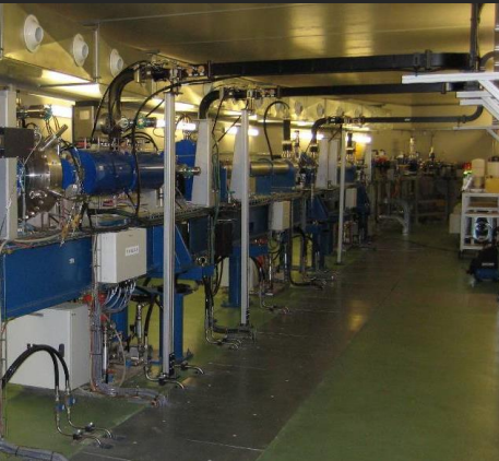
LINAC: 3GHz structure, beam acceleration to 100 MeV
