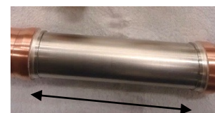
0.3 mm Stainless Steel sector For fast orbit correctors
