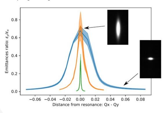
strong → skew on to increase the coupling nominal → skew off, natural coupling weak → skew on to correct the coupling
