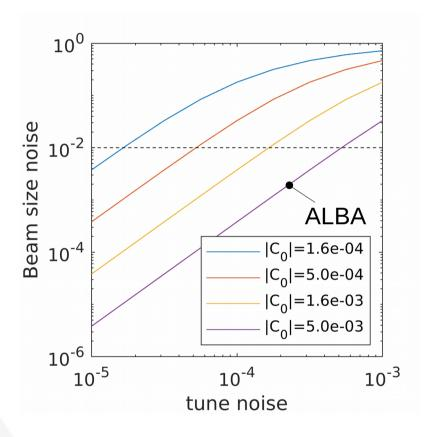
For ALBA-II, **if we work in full coupling,** we will need enough coupling strength  $|C_0|$  to produce a **small beam noise**. Typically beamlines ask for a 10% but that should include also orbit stability. to be safe we should target few times 1%.
